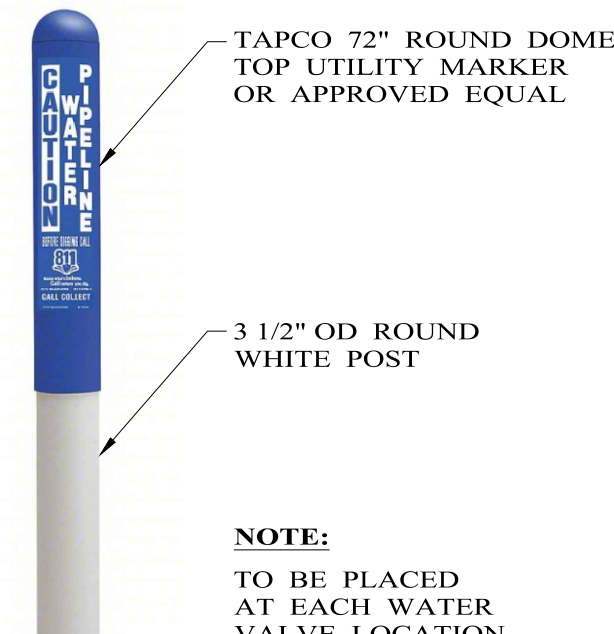
TYPICAL UTILITY/VALVE MARKER DETAIL
